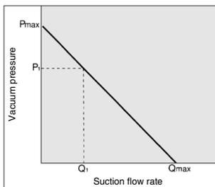
Flow rate characteristics are expressed in ejector vacuum pressure and suction flow rate. If suction flow rate changes, a change in vacuum pressure will also be expressed. Normally this relationship is expressed in ejector standard use.
